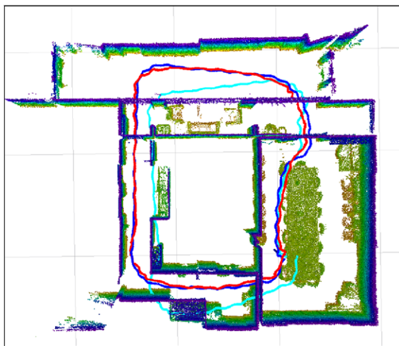
Figure 11. Accuracy comparison with ground truth in an office environment: Cyan: odometry. Red: localization. Blue: ground truth.
