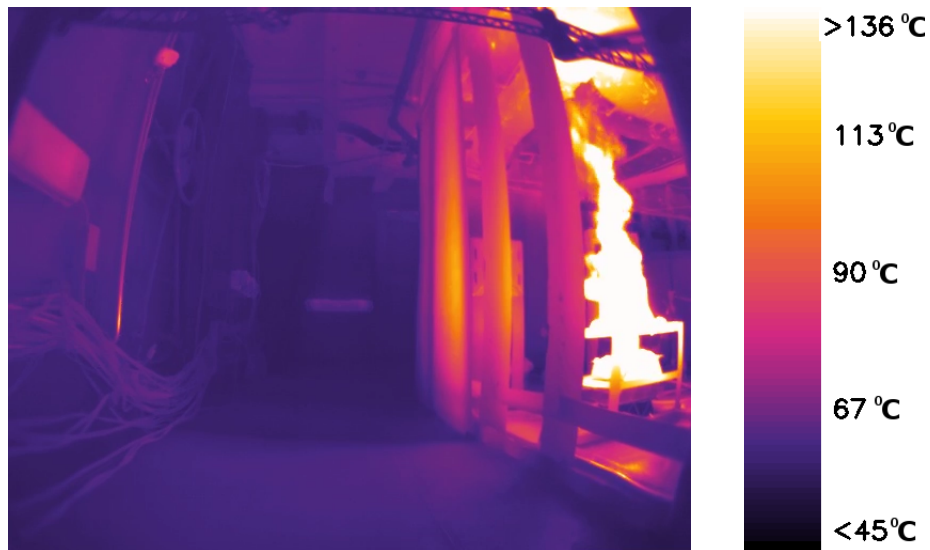
Figure 9: A colorized image output from FLIR thermal camera (Wood Fire).
