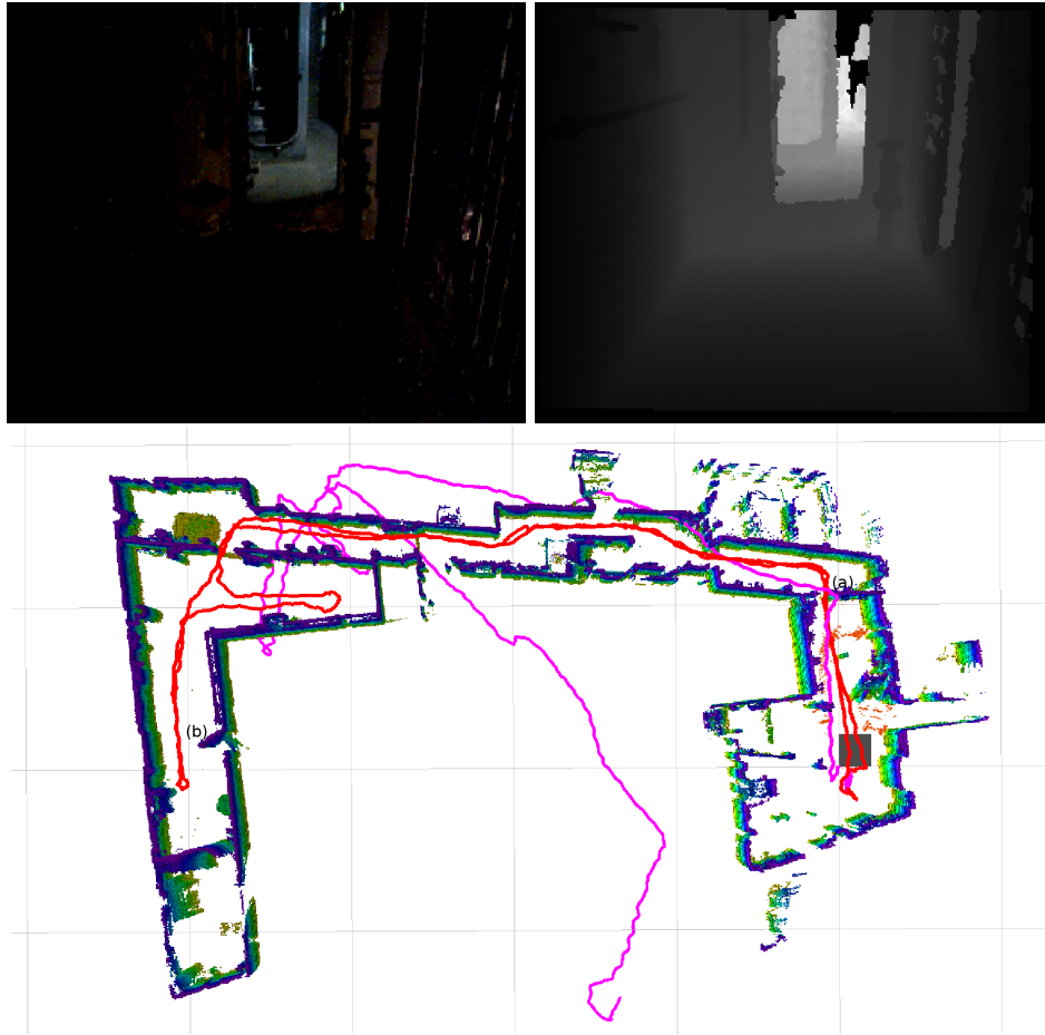
Figure 12: Localization in degraded visual environment: Pink: Odometry, Red: Localization. The bottom pictures show some snapshots of the environment. The top figure shows the odometry, localization results with the 3D octomap. Note that ceiling and ground are cropped for visualization purpose (same in the later figures).
