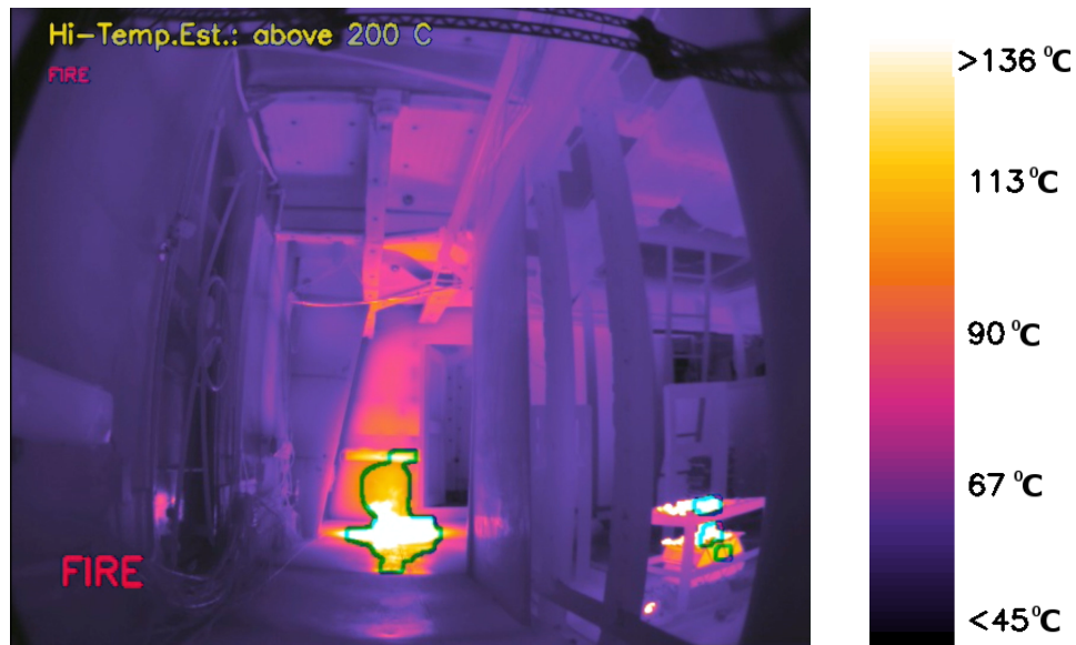
Figure 10: Fire segmentation based on temperature (Oil and Wood Fire). The detected fire sources are outlined in green.
