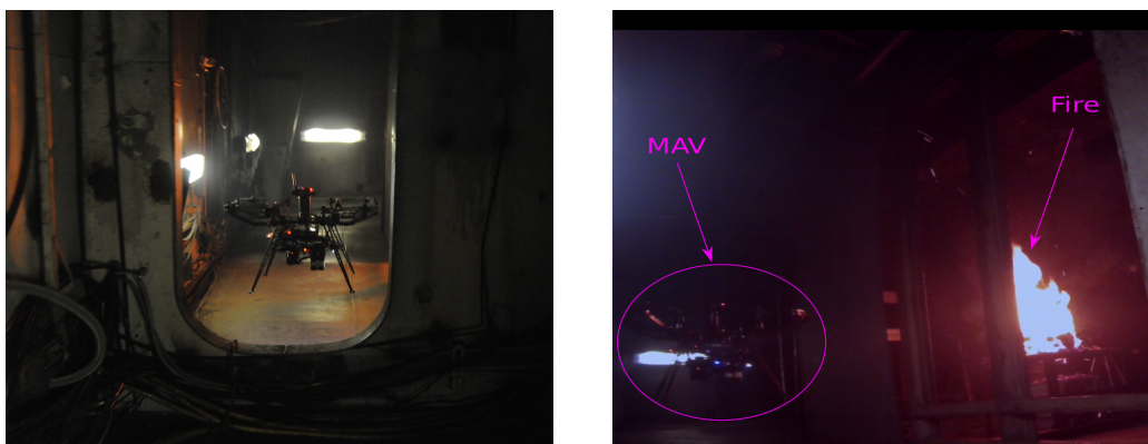
Figure 1: Autonomous MAV for fire-detection inside a ship: The left picture shows MAV's autonomous flight through doorways. The right picture shows the testing scenario with fire.
