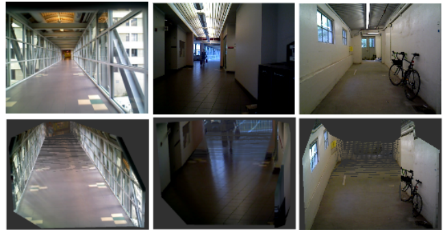
Fig. 5. 3D pop up examples from our test dataset. The first row is the raw image and the second row is the pop-up 3D model. Since our algorithm doesn't predict the ceiling plane, we manually remove points above a constant height threshold just for visualization. Since we use assumed a camera pose, the 3D model is up to scale.
