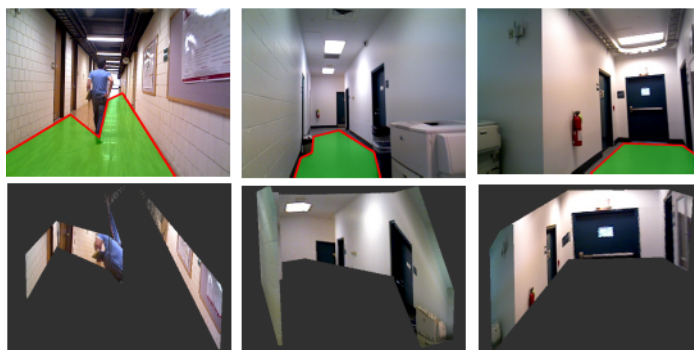
Figure 3.9: Pop-up model in a cluttered environment. Left two columns: person and printer are wrongly popped as wall. Right column: the front-facing wall in left region is wrongly popped as right-facing.
