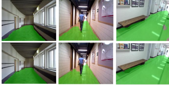
Figure 3.4: CNN prediction and CRF optimization examples on our test dataset. Row 1: CNN prediction; Row 2: CRF optimization. CNN prediction captures the general location of ground. CRF further improves the spatial consistence and captures fine details.
