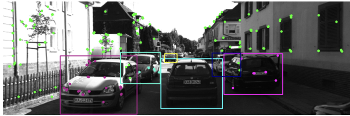
Figure 6.4: Object association in dynamic and occluded scenarios in KITTI 07. Green points are normal map points, and other color points are associated to objects with the same color. The front cyan moving car is not added as SLAM landmark as no feature point is associated with it. Points in object overlapping areas are not associated with any object due to ambiguity.
