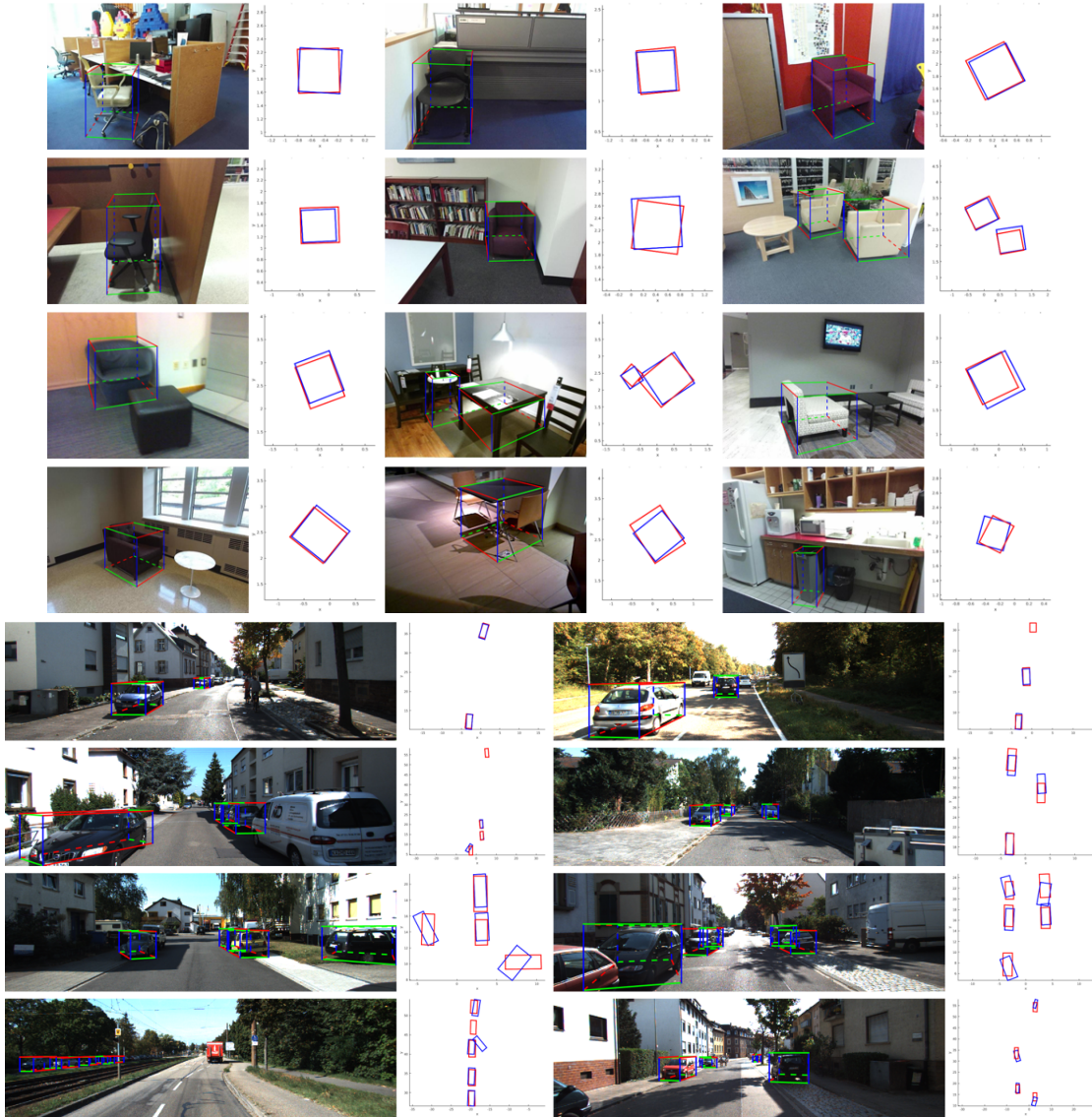
Figure 4.9: More 3D object detection examples in SUN RGBD and KITTI evaluation dataset (Single View). The top view shows the predicted cuboid (blue) and ground truth matched object (red).
